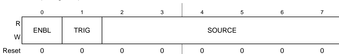
Figure 143. Channel Configuration Registers (CHCONFIG n )
