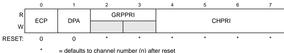
Figure 135. DMA Channel n Priority (EDMA_CPRn) Register
