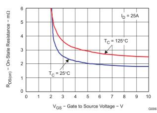
Figure 7. On Resistance vs. Gate Voltage
