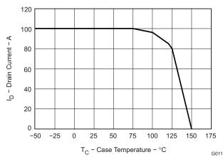
Figure 12. Maximum Drain Current vs. Temperature
