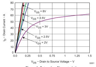
Figure 2. Saturation Characteristics
