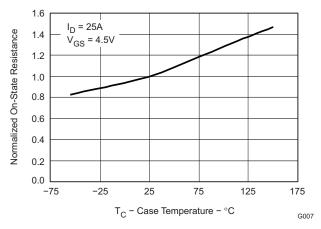
Figure 8. On Resistance vs. Temperature
