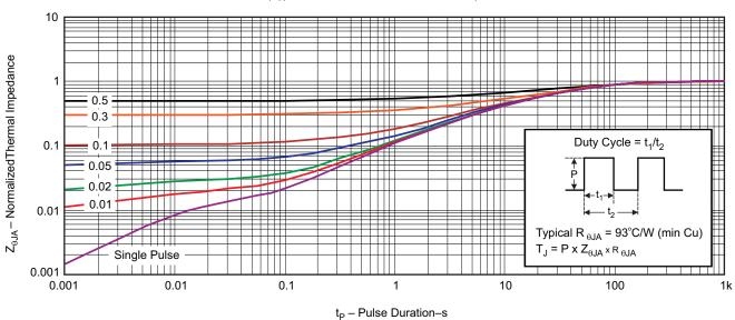
Figure 1. Transient Thermal Impedance
