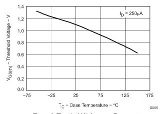
Figure 6. Threshold Voltage vs. Temperature
