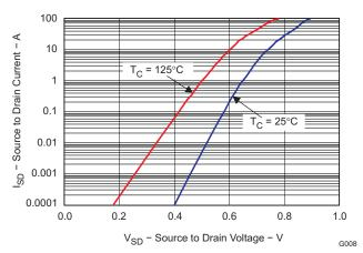
Figure 9. Typical Diode Forward Voltage
