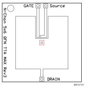
Max  $R_{\theta JA} = 48^{\circ}\text{C/W}$  when mounted on 1 in<sup>2</sup> of 2-oz. Cu.
