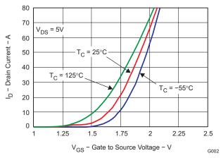
Figure 3. Transfer Characteristics
