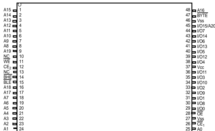
Figure 2. 48-pin TSOP I (12 × 18.4 × 1.0 mm) Top View [2, 3]
