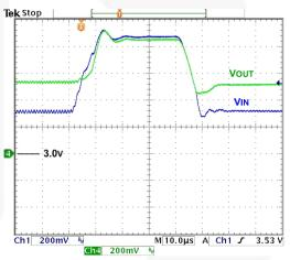
Figure 25. Line Transient, 3.0-3.6  $V_{IN}$ , 10  $\mu s$  Edge, 1,000 mA Load,  $V_{OUT}$ =3.5 V
