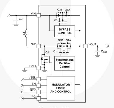
Figure 2. Block Diagram
