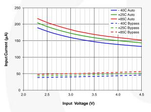
Figure 13. Quiescent Current vs. Input Voltage, Temperature and Mode, V<sub>OUT</sub>=5.0 V, Forced Bypass, OCP Active
