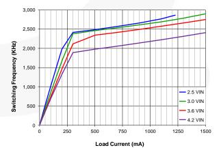
Figure 16. Frequency vs. Load Current and Input Voltage
