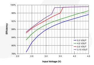
Figure 9. Efficiency vs. Input Voltage and Output Voltage, Figure 10. Efficiency vs. Input Voltage and Output Voltage, 200 mA Load
