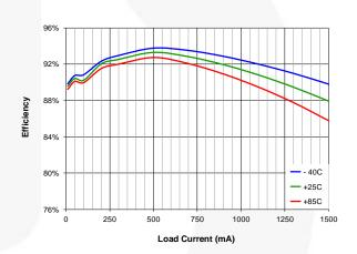
Figure 7. Efficiency vs. Load Current and Input Voltage
