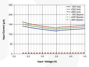
Figure 14. Quiescent Current vs. Input Voltage, Temperature and Mode,  $V_{\text{OUT}}$ =3.5 V, Forced Bypass, Low  $I_{\text{Q}}$
