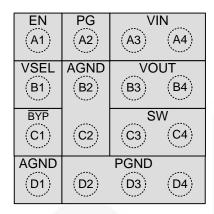
Figure 3. Top Through View (Bumps Down)
