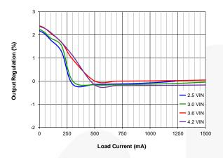
Figure 11. Output Regulation vs. Load Current and Input Voltage (Normalized to 3.6 V<sub>IN</sub>, 500 mA Load)
