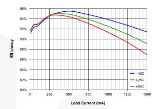
Figure 5. Efficiency vs. Load Current and Input Voltage,  $$V_{\text{OUT}}$=$3.5~\text{V}$$
