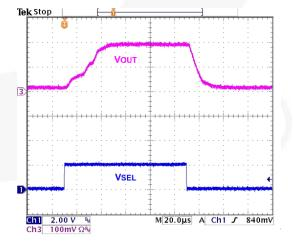
Figure. 27 Bypass Entry / Exit, Slow  $V_{IN}$  Ramp 1 ms Edge, 500 mA Load,  $V_{OUT}{=}3.5$  V, 3.2 - 3.8  $V_{IN}$
