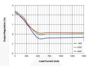
Figure 12. Output Regulation vs. Load Current and Temperature (Normalized to 3.6  $V_{IN}$ , 500 mA Load,  $T_A=25^{\circ}C$ )
