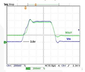
Figure 23. Transient Overload, 500-1950 mA, 100 ns Edge,  $\rm V_{IN}{=}3~V,~V_{OUT}{=}3.5~V$
