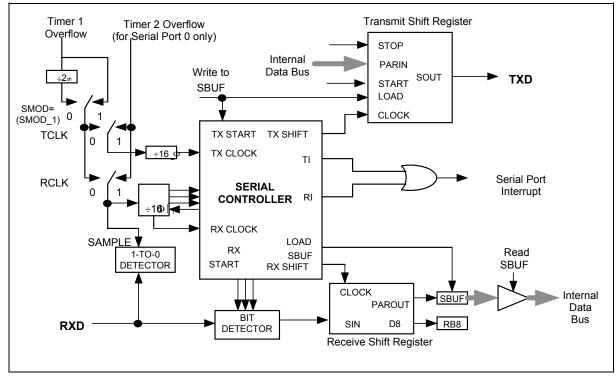
Figure 21: Serial Port Mode 1
