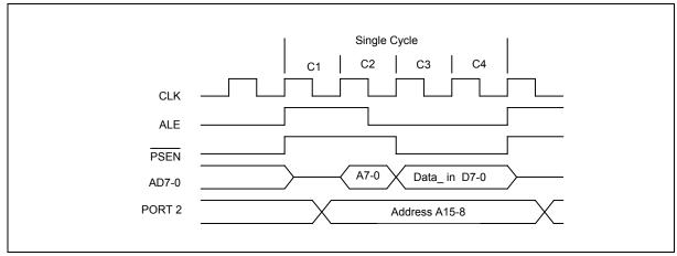
Figure 3. Single Cycle Instruction Timing
