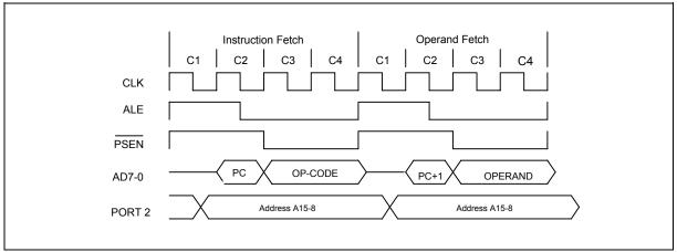
Figure 4. Two Cycle Instruction Timing
