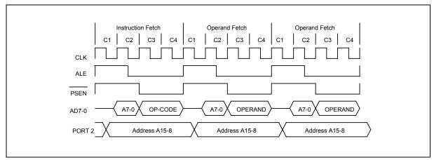
Figure 5. Three Cycle Instruction Timing
