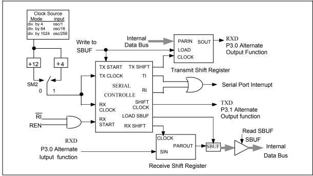
Figure 20. Serial Port Mode 0
