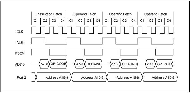
Figure 6. Four Cycle Instruction Timing
