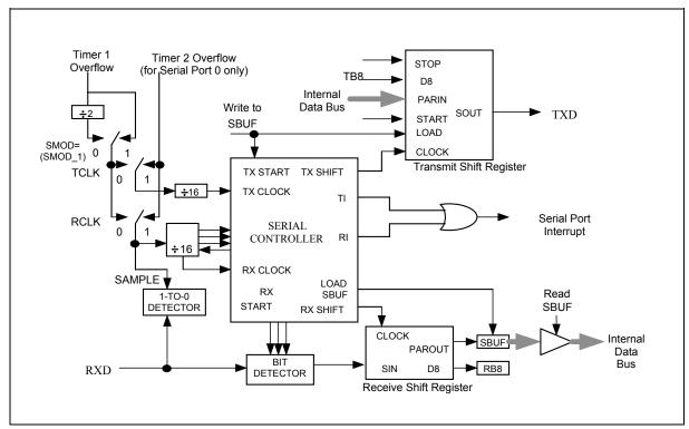
Figure 23: Serial Port Mode 3
