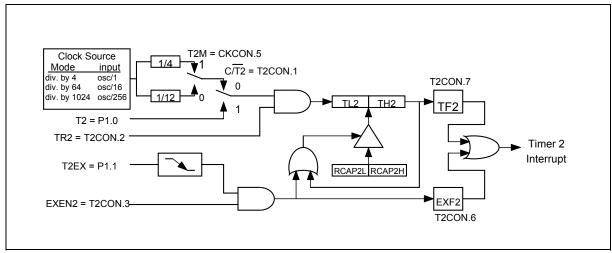
Figure 15. 16-Bit Auto-reload Mode, Counting Up
