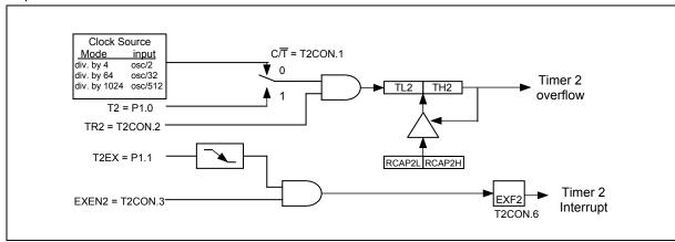
Figure 17. Baud Rate Generator Mode
