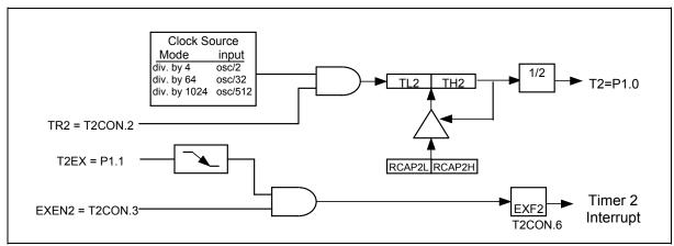
Figure 18. Programmable Clock-Out Mode
