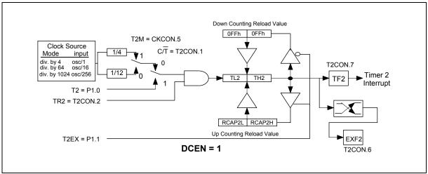
Figure 16. 16-Bit Auto-reload Up/Down Counter
