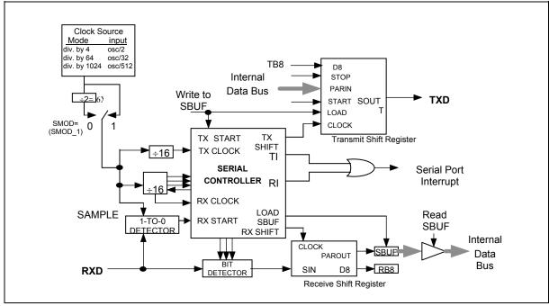
Figure 22. Serial Port Mode 2
