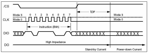
Figure 15. Deep Power-down Instruction Sequence Diagram
