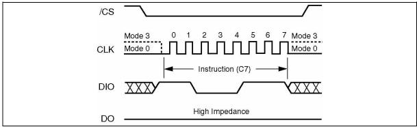
Figure 14. Chip Erase Instruction Sequence Diagram
