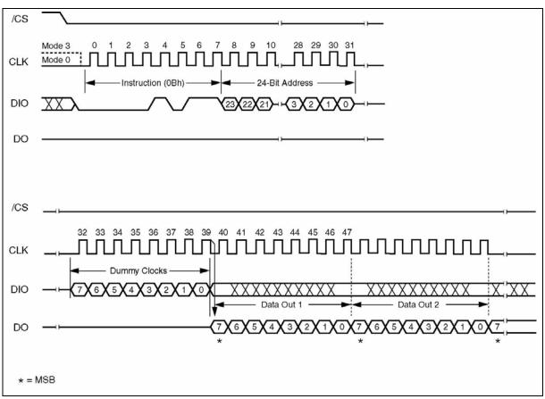
Figure 9. Fast Read Instruction Sequence Diagram
