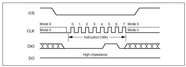
Figure 4. Write Enable Instruction Sequence Diagram
