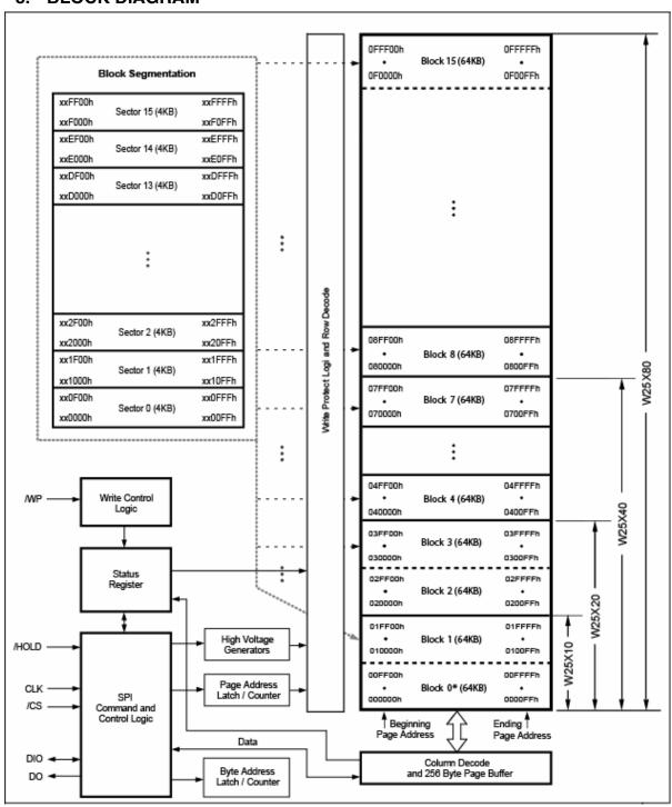
Figure 2. W25X10, W25X20, W25X40 and W25X80 Block Diagram
