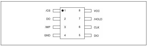
Figure 1a. W25X10, W25X20 and W25X40 Pin Assignments, 8-pin SOIC (Package Code SN)
