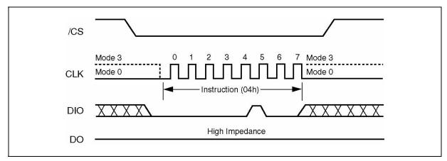
Figure 5. Write Disable Instruction Sequence Diagram
