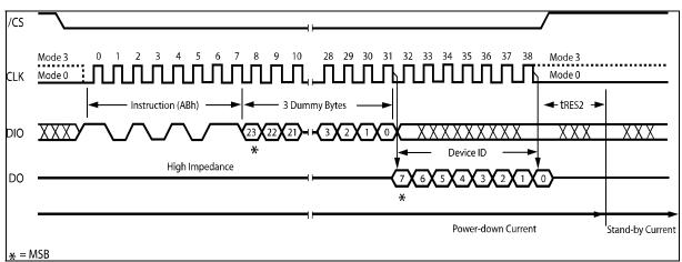
Figure 17. Release Power-down / Device ID Instruction Sequence Diagram
