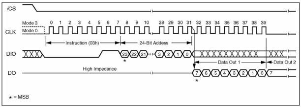
Figure 8. Read Data Instruction Sequence Diagram
