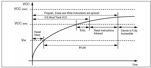
Figure 20. Power-up Timing and Voltage Levels
