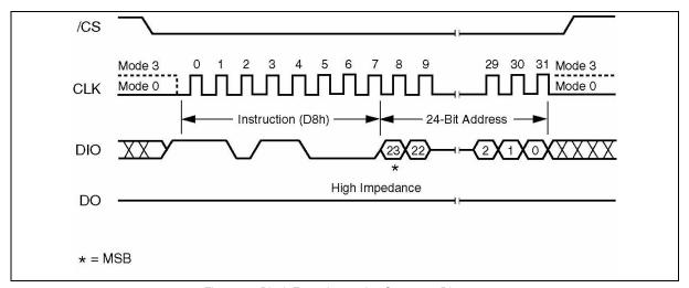
Figure 13. Block Erase Instruction Sequence Diagram
