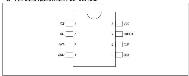
Figure 1c. W25X10, W25X20, W25X40 and W25X80 Pin Assignments, 8-pin PDIP (Package Code DA)
