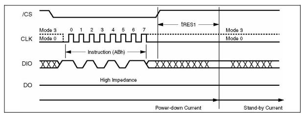
Figure 16. Release Power-down Instruction Sequence
