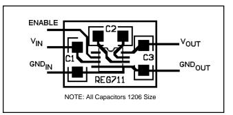
FIGURE 4. Suggested PCB Design for Minimum Ripple.
