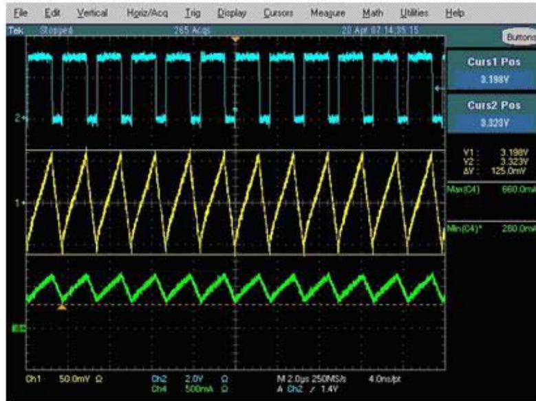
Figure 11. Electrolytic 100 \mu F (Ripple Too High)
