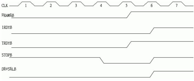
Figure 14. Target Initiated Termination - Disconnect
