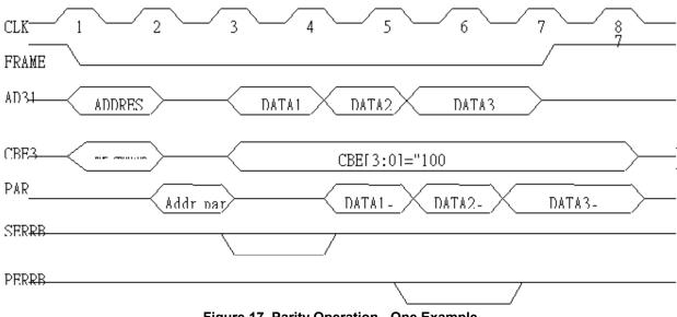
Figure 17. Parity Operation - One Example
