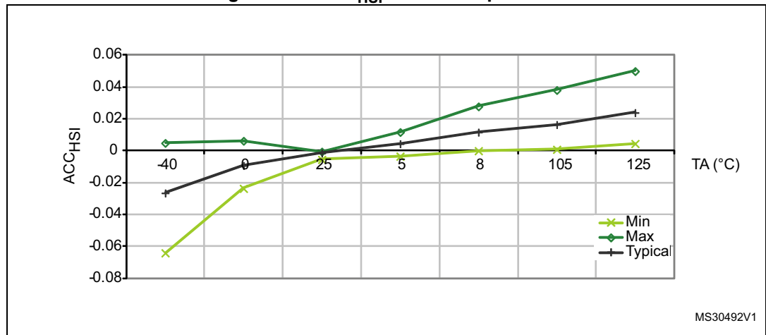
Figure 27. LACC_{HSI} versus temperature
