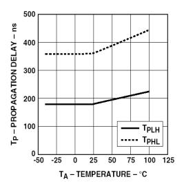
Figure 12. Propagation Delay vs. Temperature.
