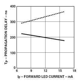
Figure 11. Propagation Delay vs. I<sub>F</sub>.
