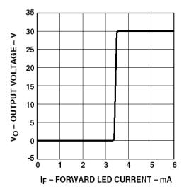
Figure 15. Transfer Characteristics.
