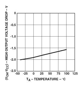
Figure 1. V<sub>OH</sub> vs. Temperature.
