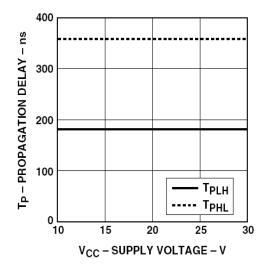
Figure 10. Propagation Delay vs. V<sub>CC</sub>.
