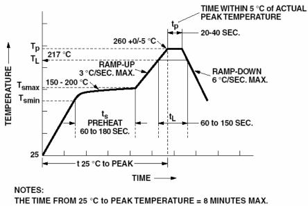
$T_{smax} = 200 \ ^{\circ}C, T_{smin} = 150 \ ^{\circ}C$
