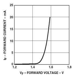
Figure 16. Input Current vs. Forward Voltage.
