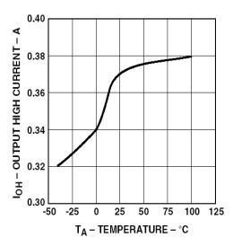
Figure 2. I<sub>OH</sub> vs. Temperature.
