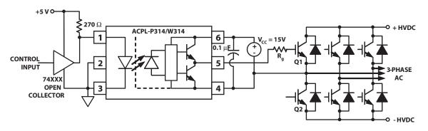
Figure 19. Recommended LED Drive and Application Circuit for ACPL-P314/W314
