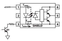
Figure 24. Not Recommended Open Collector Drive Circuit.
