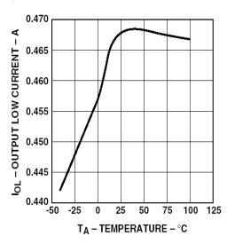
Figure 5. I<sub>OL</sub> vs. Temperature.
