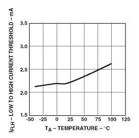
Figure 9. IFLH vs. Temperature.
