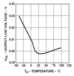
Figure 4. V<sub>OL</sub> vs. Temperature.
