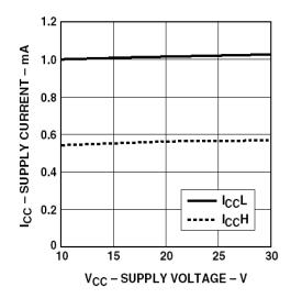
Figure 8. I<sub>CC</sub> vs. V<sub>CC</sub>.
