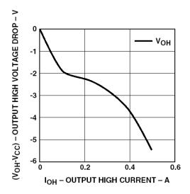
Figure 3. V<sub>OH</sub> vs. I<sub>OH</sub>.
