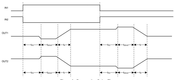
Figure 6. Propagation Delay Time
