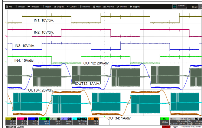
Figure 50. Stepper Motor Half-Step Operation With Off-State as Brake
