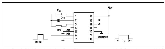
A positive MASTER RESET pulse clears the counter and latch. The Output goes high and keeps up till the number of pulses, selected by A and B, are counted. This circuit is retriggerable and is as accurate as the input frequency. If a
