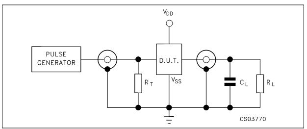
$C_L$  = 50pF or equivalent (includes jig and probe capacitance)  $R_L$  = 200K $\Omega$   $R_T$  =  $Z_{OUT}$  of pulse generator (typically 50 $\Omega$ )
