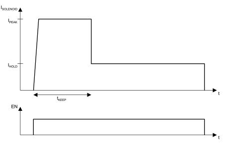
Figure 2. Typical Current Waveform Through the Solenoid
