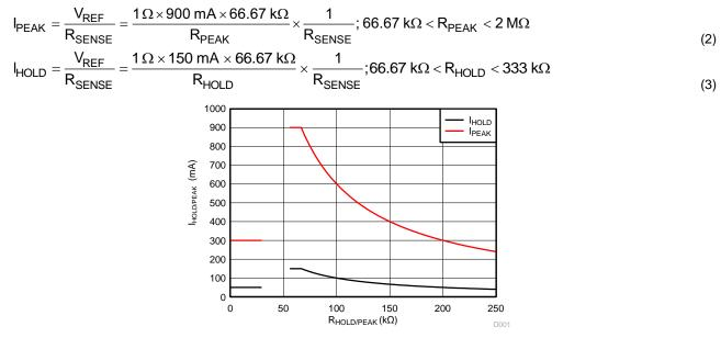
Figure 4. I<sub>PEAK</sub> and I<sub>HOLD</sub> settings for R<sub>SENSE</sub> = 1  $\Omega$
