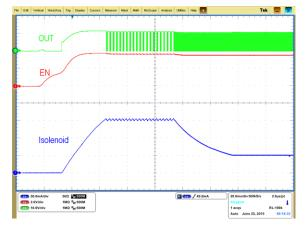
Figure 1. Solenoid Current, EN, and PWM vs Time
