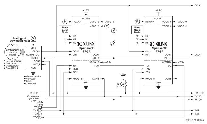
Figure 61: Daisy-Chaining using Slave Serial Mode
