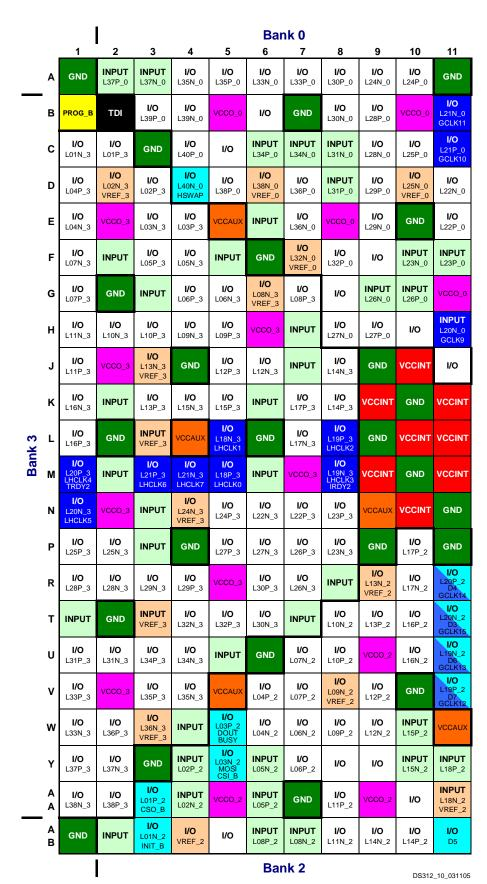
Figure 10: FG484 Package Footprint (top view)
