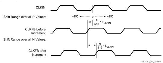
Figure 41: Phase Shifter Waveforms
