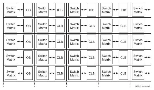
Figure 46: Array of Interconnect Tiles in Spartan-3E FPGA
