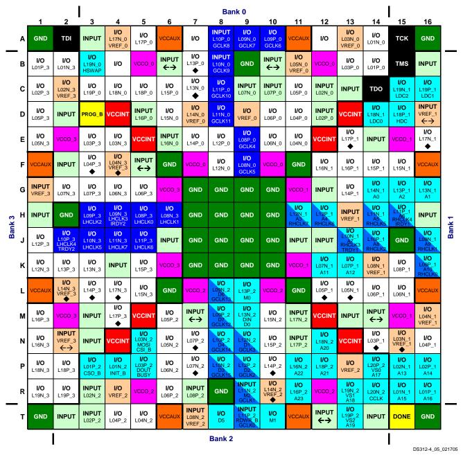
Figure 7: FT256 Package Footprint (top view)
