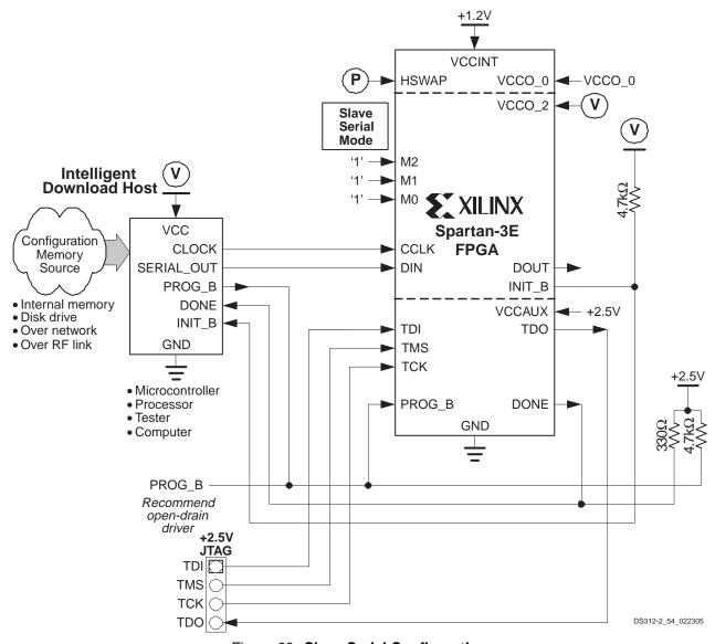
Figure 60: Slave Serial Configuration
