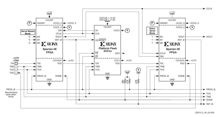
Figure 49: Daisy-Chaining from Master Serial Mode
