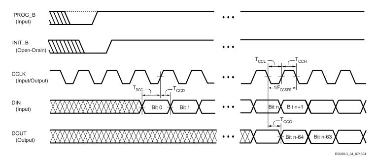
Figure 4: Waveforms for Master and Slave Serial Configuration
