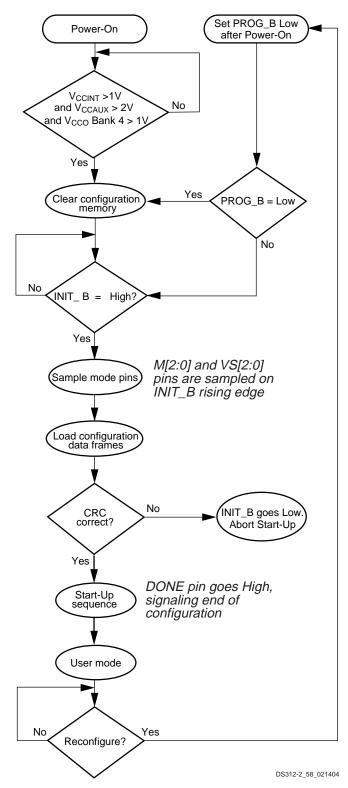
Figure 64: General Configuration Process
