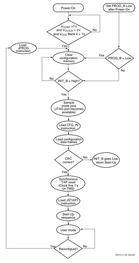
Figure 65: Boundary-Scan Configuration Flow Diagram
