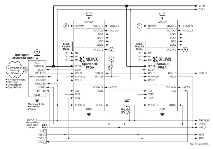
Figure 59: Daisy-Chaining using Slave Parallel Mode
