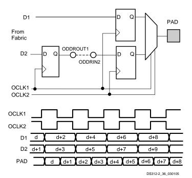
Figure 7: Output DDR Using Spartan-3E Cascade Feature
