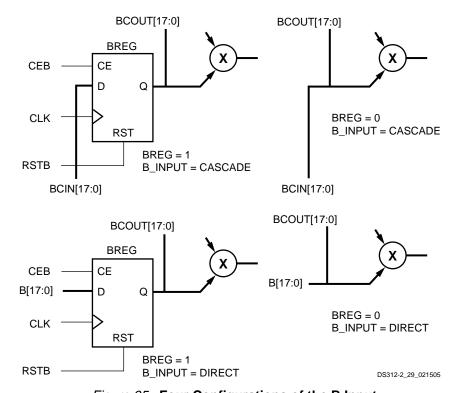
Figure 35: Four Configurations of the B Input
