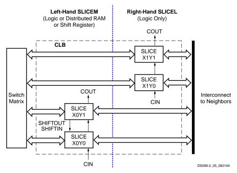
Figure 13: Arrangement of Slices within the CLB
