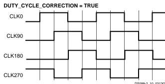
Figure 40: Characteristics of the DLL Clock Outputs
