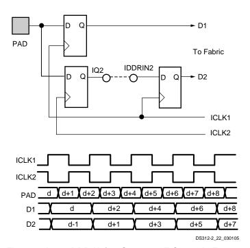
Figure 5: Input DDR Using Spartan-3E Cascade Feature
