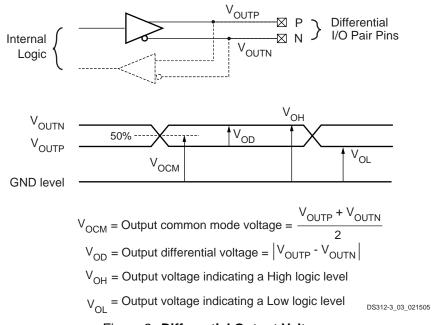
Figure 2: Differential Output Voltages
