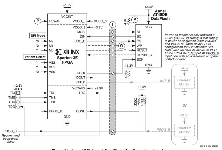
Figure 51: Atmel SPI-based DataFlash Configuration Interface
