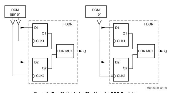
Figure 3: Two Methods for Clocking the DDR Register
