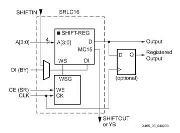
Figure 25: Logic Cell SRL16 Structure
