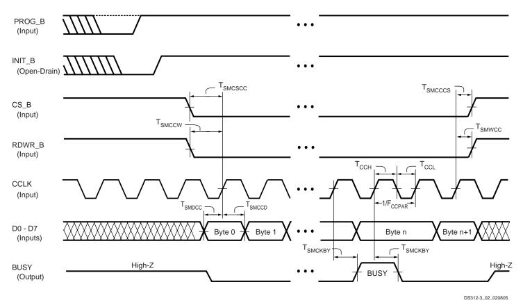
It is possible to abort configuration by pulling CS\_B Low in a given CCLK cycle, then switching RDWR\_B Low or High in any subsequent cycle for which CS\_B remains Low. The RDWR\_B pin asynchronously controls the driver impedance of the D0 - D7 bus. When RDWR\_B switches High, be careful to avoid contention on the D0 - D7 bus.
