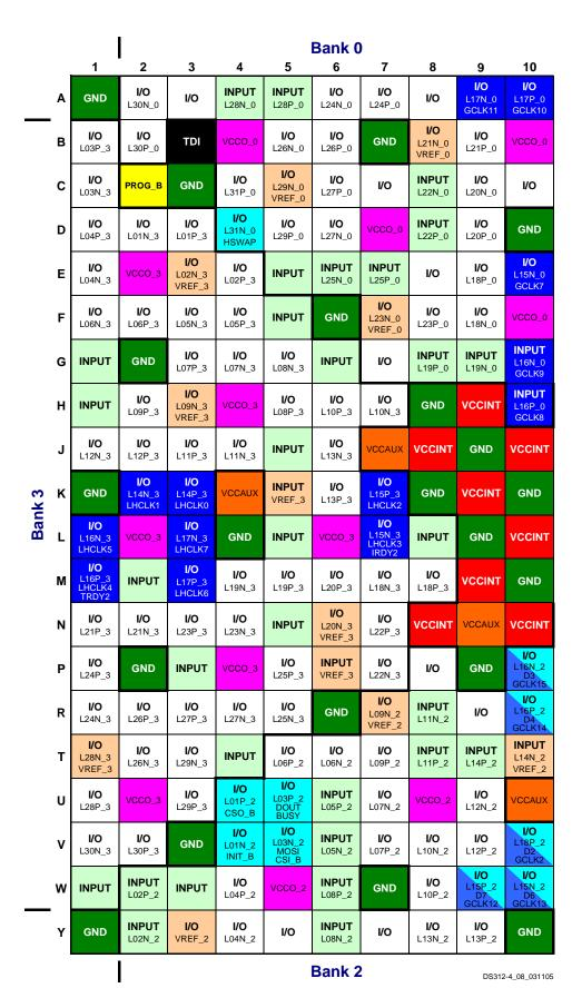
Figure 9: FG400 Package Footprint (top view)
