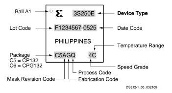
Figure 4: Spartan-3E CP132 and CPG132 Example Package Marking
