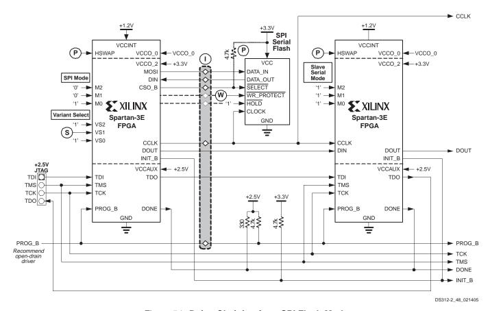
Figure 54: Daisy-Chaining from SPI Flash Mode
