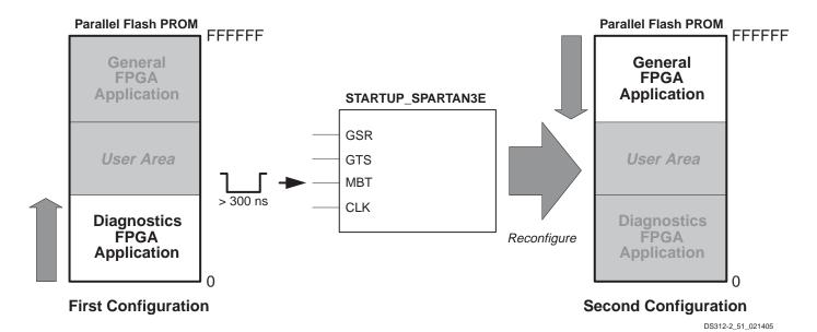
Figure 57: Use MultiBoot to Load Alternate Configuration Images
