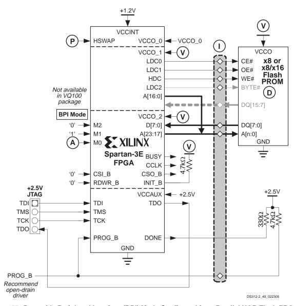
Figure 55: Byte-wide Peripheral Interface (BPI) Mode Configured from Parallel NOR Flash PROMs
