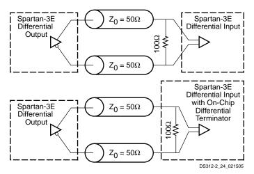
Figure 8: Differential Inputs and Outputs
