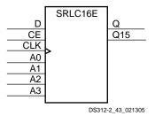
Figure 26: SRL16 Shift Register Component with Cascade and Clock Enable
