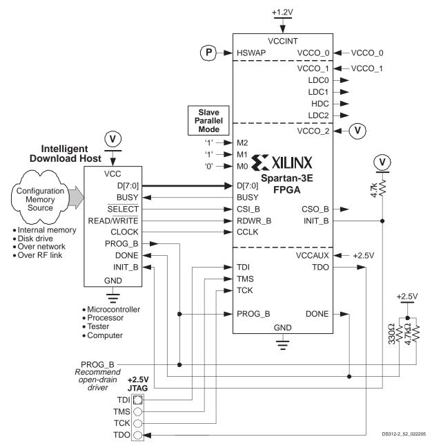
Figure 58: Slave Parallel Configuration Mode
