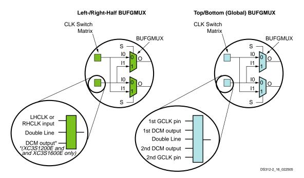
Figure 43: Clock Switch Matrix to BUFGMUX Pair Connectivity
