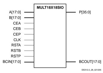
Figure 34: MULT18X18SIO Primitive
