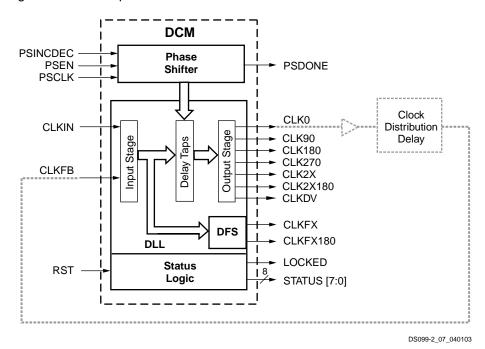
Figure 37: DCM Functional Blocks and Associated Signals
