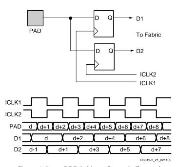
Figure 4: Input DDR (without Cascade Feature)
