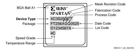
Figure 3: Spartan-3E BGA Example Package Marking
