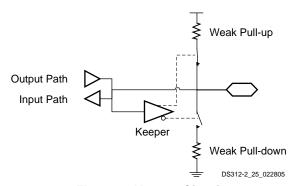
Figure 9: Keeper Circuit
