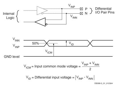
Figure 1: Differential Input Voltages
