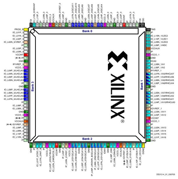
Figure 4: TQ144 Package Production Footprint (top view)
