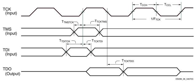
Figure 6: JTAG Waveforms
