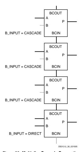
Figure 36: Multiplier Cascade Connection
