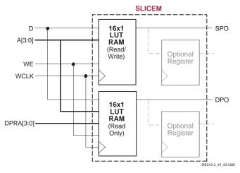
Figure 23: RAM16X1D Dual-Port Usage
