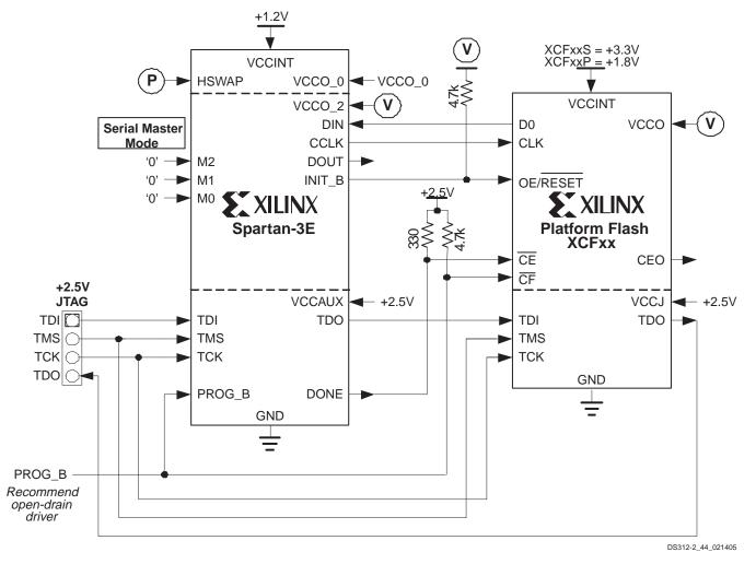
Figure 48: Master Serial Mode using Platform Flash PROM
