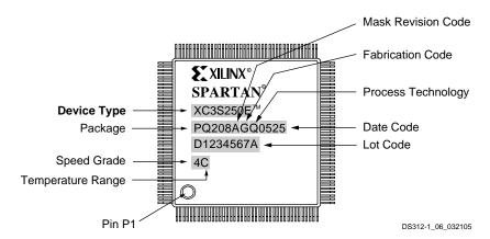
Figure 2: Spartan-3E QFP Example Package Marking
