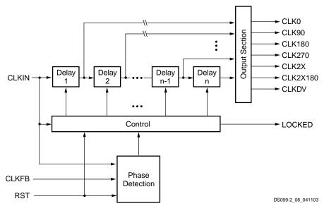
Figure 38: Simplified Functional Diagram of DLL
