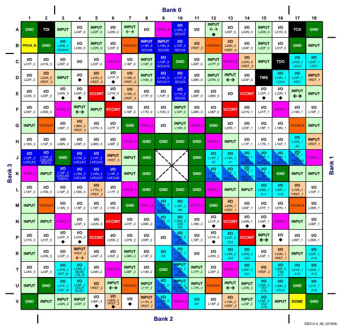
Figure 8: FG320 Package Footprint (top view)
