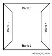
Figure 10: Spartan-3E I/O Banks (top view)
