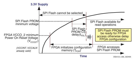
Figure 52: SPI Flash PROM/FPGA Power-On Timing if 3.3V Supply is Last in Power-On Sequence
