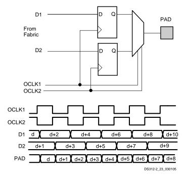
Figure 6: Output DDR (without Cascade Feature)
