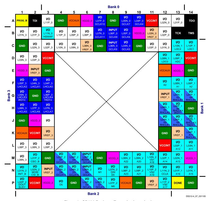
Figure 3: CP132 Package Footprint (top view)
